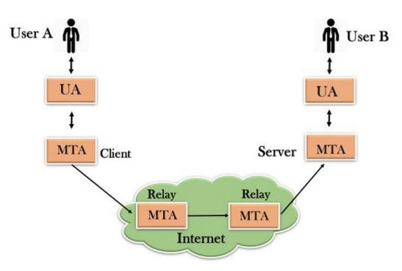
The relaying system without TCP/IP protocol can also be used to send the emails to users, and this is achieved by the use of the mail gateway. The mail gateway is a relay MTA that can be used to receive an email.
