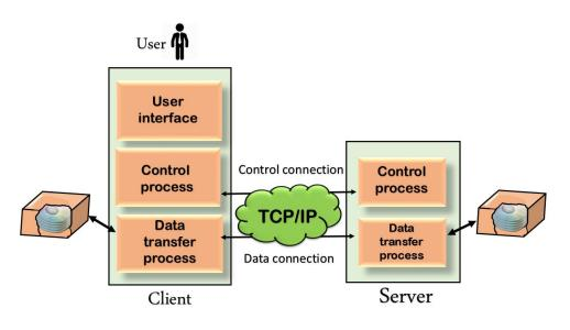
The above figure shows the basic model of the FTP. The FTP client has three components: the user interface, control process, and data transfer process. The server has two components: the server control process and the server data transfer process.
