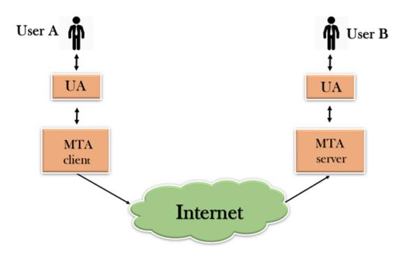
SMTP allows a more complex system by adding a relaying system. Instead of just having one MTA at sending side and one at receiving side, more MTAs can be added, acting either as a client or server to relay the email.
